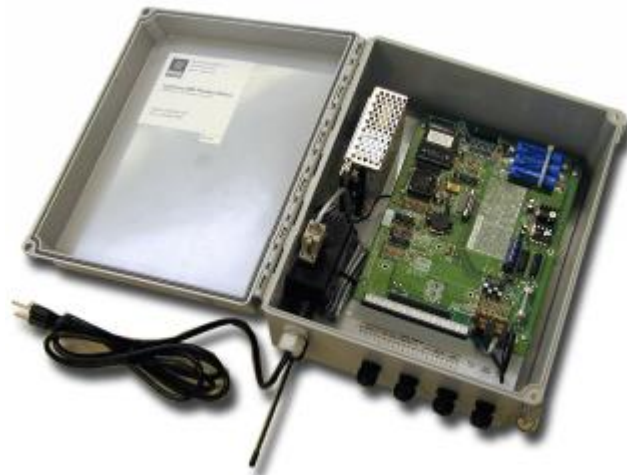
Figure 2-1: Control module's system board[4]
